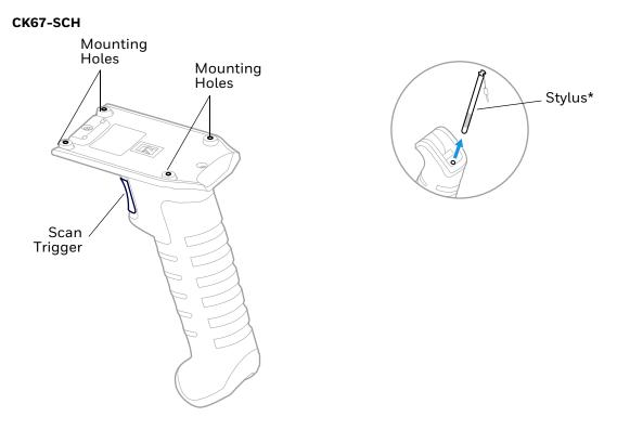
\*For information on ordering a replacement stylus, see the Accessory Guide for your device, available for download at automation.honeywell.com.
