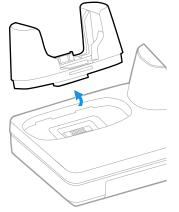
4. Insert the new cup tilted slightly towards the front of the base.
