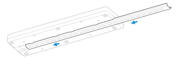
2. Secure the DIN rail to the flat surface with the hardware.
