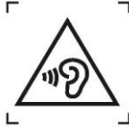
Figure 1 – Warning label (IEC 60417-6044)
