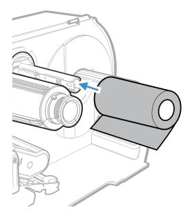
**Note:** For ribbon that has the ink wound out, place the ribbon on the ribbon supply hub with the ribbon wound clockwise. For ribbon that has the ink wound in, place the ribbon on the ribbon supply hub with the ribbon wound counterclockwise.
