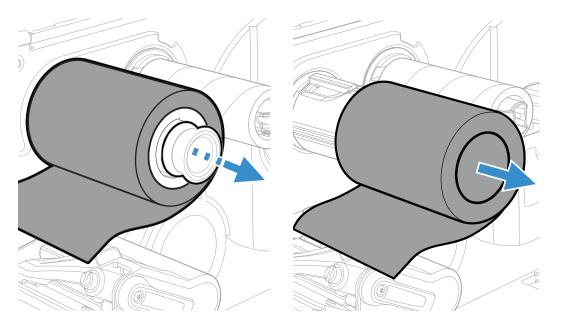
**Note:** Do not pull the ribbon release knob if you do not want to remove the used ribbon as this will cause difficulty to remove ribbon when full.
