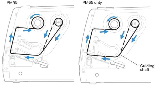
5. Turn the ribbon take-up collapsible core counterclockwise until the ribbon stays tight and runs wrinkle-free through the print mechanism.
