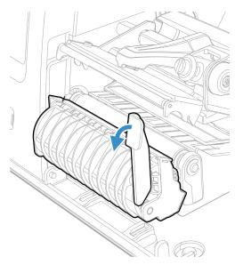
4. Load a media roll onto the media supply hub. Adjust the edge guide and dancer guide to hold the media in place.
