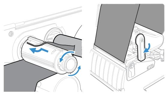
6. Turn the printhead lever clockwise to lock the printhead in position.
