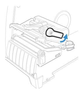
3. Load the media roll onto the media supply hub.
