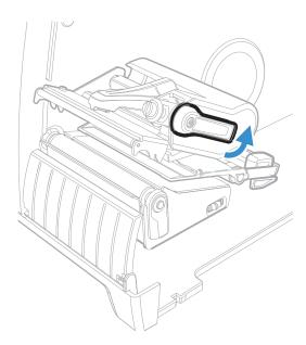
3. Feed media through the slot in the back of the printer (or from the slot in the bottom of the printer) and route it through the print mechanism.
