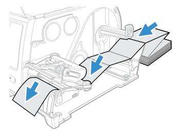
4. Turn the printhead lift lever clockwise to close the printhead. The printer performs the action defined by the Head Down Action setting (Smart calibration).
