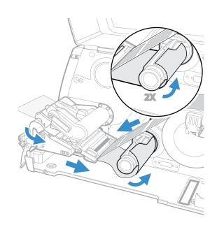
Route the liner around collapsible core
