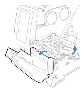
4. Load a media roll onto the media supply hub.
