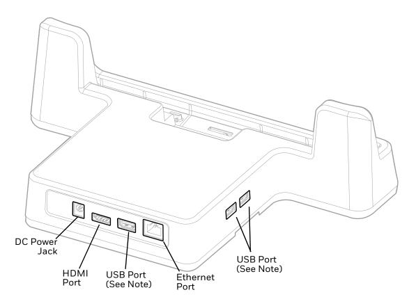
**Note:** The display dock supports USB direct connections only. The dock does not support USB hub connections, including keyboards with USB port(s).
