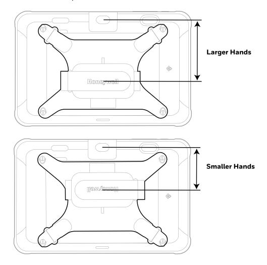
1. Align the holes in the hand strap with the holes on the back of the tablet.
