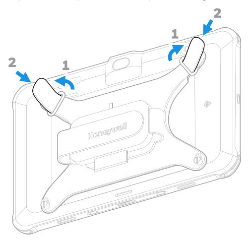
2. Fold the hand strap back to reveal the battery cover.
