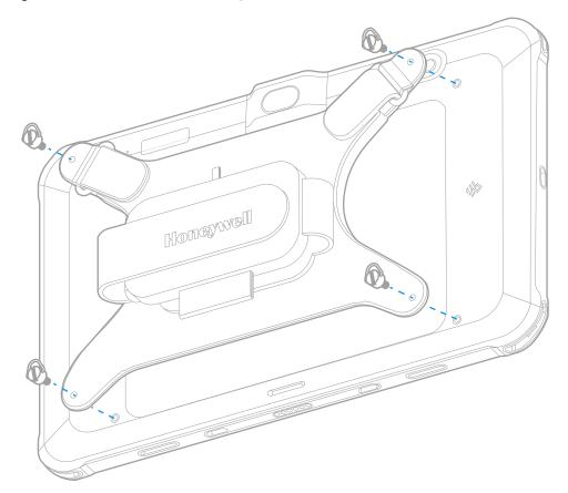
2. Insert a D-ring thumb screw into each hole and hand tighten.
